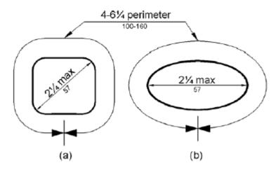
Figure 505.7.2 Handrail Non-Circular Cross Section
