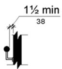
Figure 505.5 Handrail Clearance
