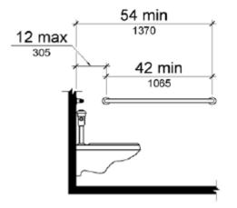
Figure 604.5.1 Side Wall Grab Bar at Water Closets
