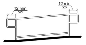
Figure 505.10.1 Top and Bottom Handrail Extension at Ramps
