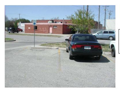
No access aisle. Parking space is required to be 132" wide with a 60" Access aisle.
