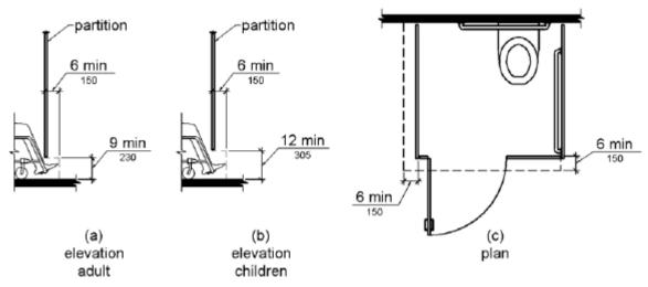
Figure 604.8.1.4 Wheelchair Accessible Toilet Compartment Toe Clearance
