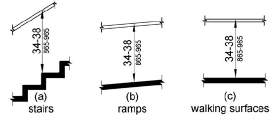
Figure 505.4 Handrail Height
