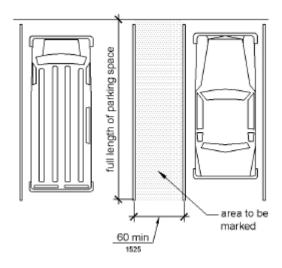
Figure 502.3 Parking Space Access Aisle
