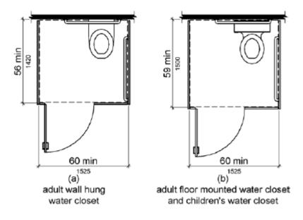
Figure 604.8.1.1 Size of Wheelchair Accessible Toilet Compartment
