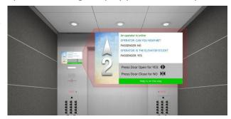
ASME A17.1 Chapter 2 Section 2.27.1.1.3—The code also requires a means to display video to observe passengers at any location on the car floor, to authorized personnel for entrapment assessment.
