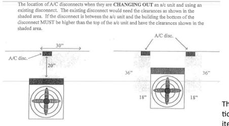
The A/C unit is NOT ALLOWED to be positioned back in its existing location if these items cannot be met.
