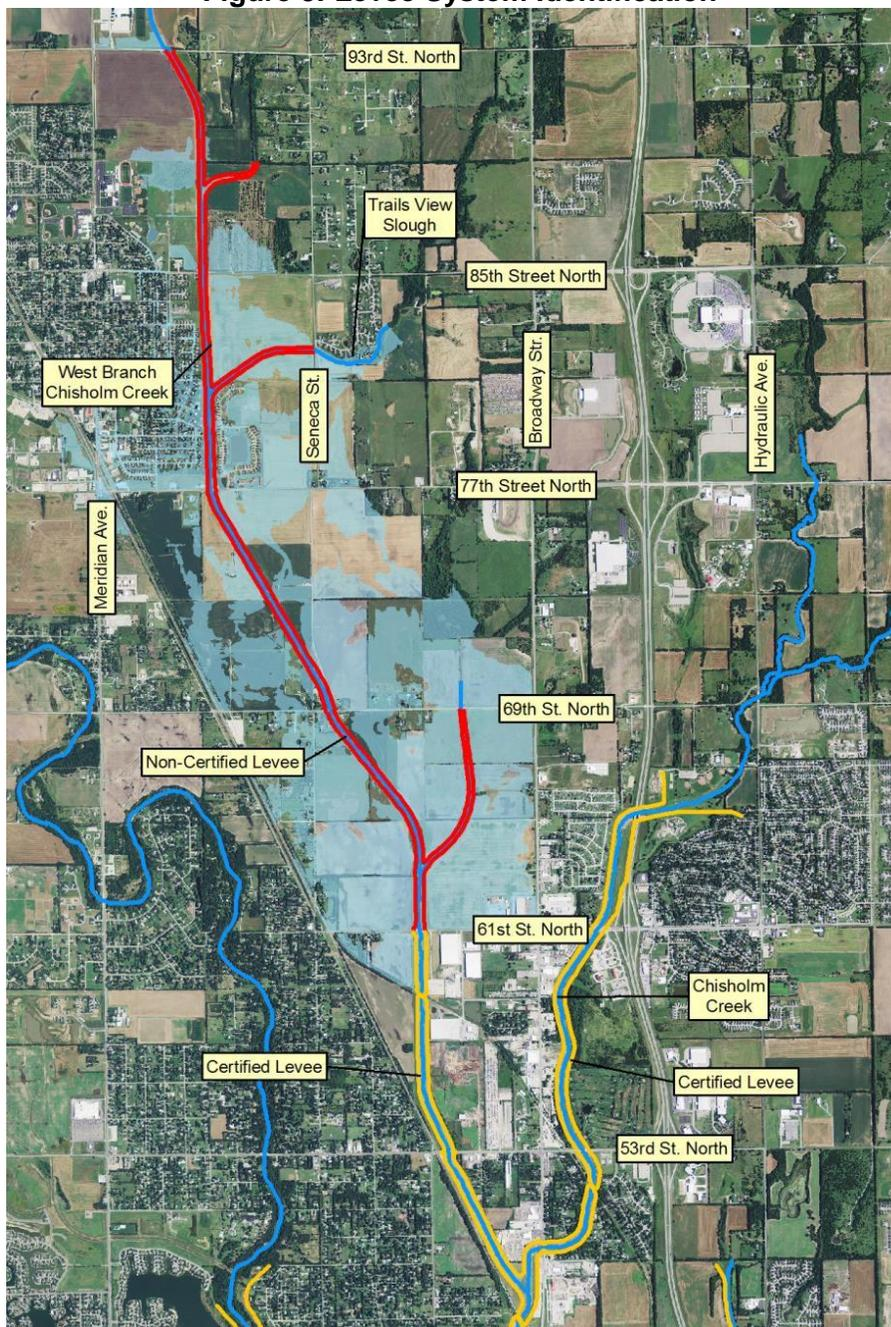
Hydrologic and hydraulic models previously developed during the Sedgwick County DFIRM project and Wichita Levee Certification project were used as the basis for this assessment. The hydrologic analysis was performed using detailed inputs into the HEC-HMS software for multiple events. Specifically, the events analyzed were the 50-, 20-, 10-, 4-, 2-, 1-, and 0.2-percent chance exceedance events. The hydrologic analysis was performed for three scenarios:
