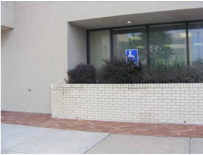
**EXISTING CONDITION:** Upright sign that designates accessible parking is not visible due to landscaping. ADAAG requires accessible parking spaces to have upright signage that is located so that it can be seen with a vehicle parked in the space.
