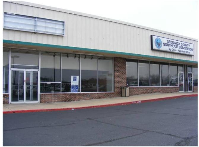
If accessible parking is provided at this location, provide a **new curb cut** in front of the main entry doors. Ensure that the path of travel from accessible parking to the facility entrance does not have cross slopes beyond 2% (as discussed above).
