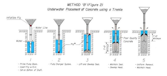
**Method B (Figure 2):** Use a tremie tube, with a pig separating the ground water and concrete, to place concrete into the shaft. Once the tremie tube is resting on the bottom of the shaft, install the pig just below the hopper in the top of the tremie tube. Fully charge the tremie tube and hopper (forcing the pig to the bottom of the tremie tube), then raise the tremie tube by 1 tremie diameter and seal the discharge end of the tremie tube with the fresh concrete.
