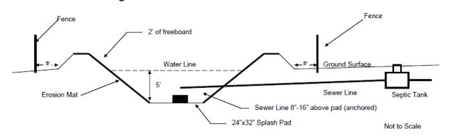
A 1,000 gallon septic tank will need to be installed in line before the lagoon and will need risers to grade. (Keep in mind that you will now have some additional fall coming to consider thru the septic tank.) If it will be a pressurized system then a 2 chamber tank will be needed.
